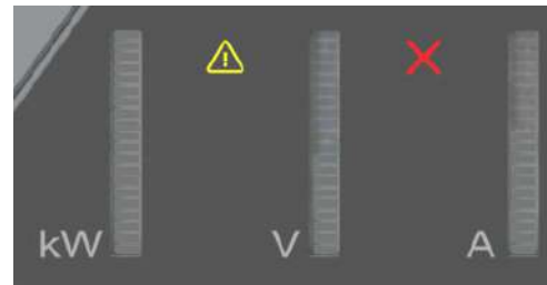
Figure 6-14: Trip/Fault Shutdown Indicator (front panel)
