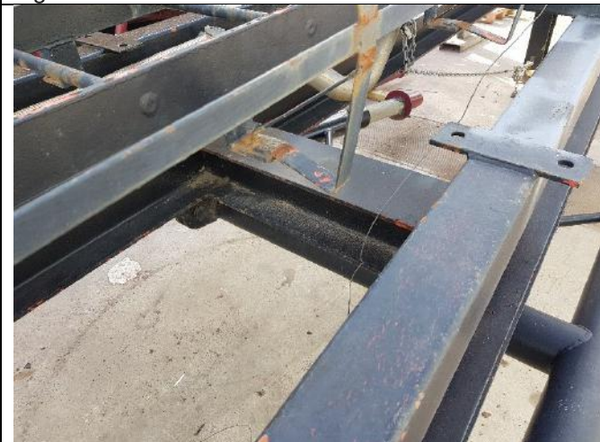
Figure.23 A-Frame Support Bracing
